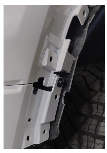
Unbolt the rear of plastic fascia, also detach the grille by removing the plastic shroud and hardware. Undo all wiring and check for connections before removing the bumper.
