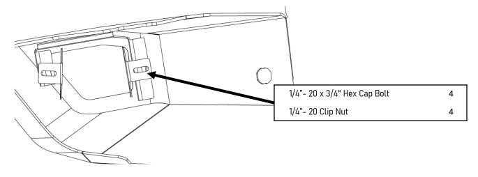
Relocate the OEM sensors to the provided brackets using 1/4" hardware. Secure to the body using the OEM hardware and locations. (L-Driver & R-Passenger).
