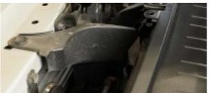
Remove the hardware for the front of the fender liner. Once removed pull the lower fender trim to access the screw and push pins behind. Undo the remaining hardware along the underside edges. Check for any remaining hardware before removing the bumper. Pull the assembly from the vehicle undoing clips in the process.
