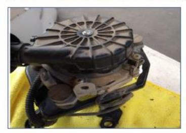
Mount the Air Pump to the bracket using the OEM hardware and attach to the body panel bracket inside the grill area. Mount the bracket using the provided hardware
