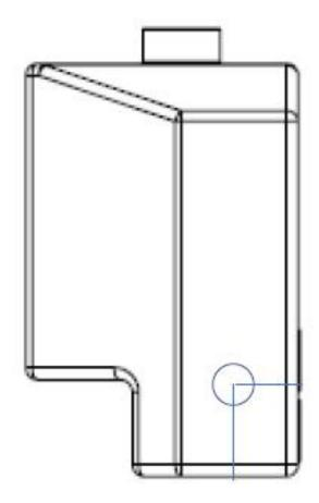
Drill in location for hose attachment. Drill to size. 3" from the bottom and 1 1/4" from the side
