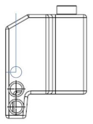
Drill in location for plug attachment. Drill to size. 6 3/4" from the top and 1 1/4" from the side
