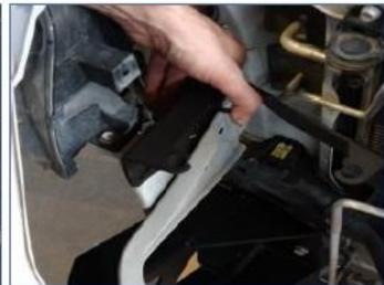
Disconnect all associated washer kit electrical and tube connections. Relocate to the air pump and reroute all connections to the area where the new washer kit will be installed
