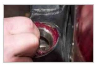
Place the washer into the swing arm, then insert the nut over the bolt. Tighten the nut using a 36mm socket. Don't over tighten to prevent binding.
