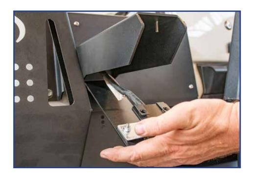
Secure and tighten with provided allen head bolts.
