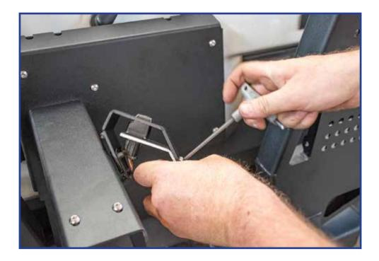
You will also need to attach two clip nuts (see photo below where the right hand is) to the bottom camera plate. (Also see photo in step 27 where the two clip nuts are attached)
