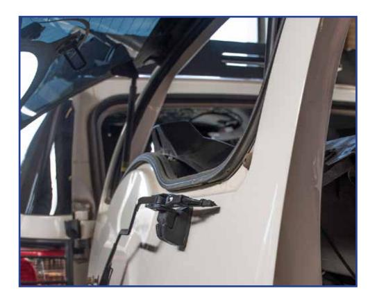
Once the plastic door panel is removed and the rear door exposed, you will need to pop these small white caps off in order to pull the seal to access the wiring. We're now prepped for wiring install later in the guide in step 18.
