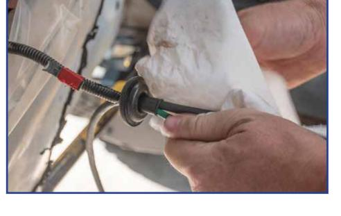
Your new wire that you fed through the rubber door grommit should be able to reach the circle highlighted on the left where we attached two red wire taps in Step 20 and out through the circle highlighted on the right side where it feeds back through the center opening for the rubber grommit. This new wire will connect to the new license plate leds on the front side of door.
