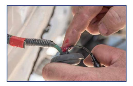
Pull the new wire through the rubber grommit until the new wire is roughly even with the stock camera wire plug. Test fit for length to make sure you can reach the red taps that were installed in steps
