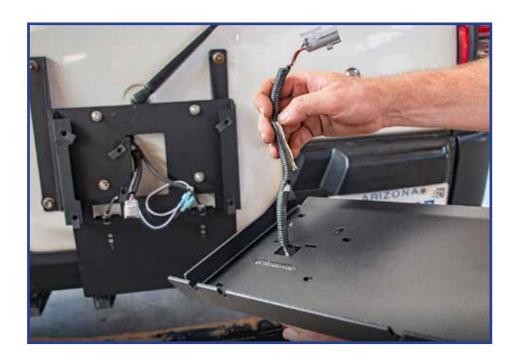
Attach and secure the camera connector to its opposite end
