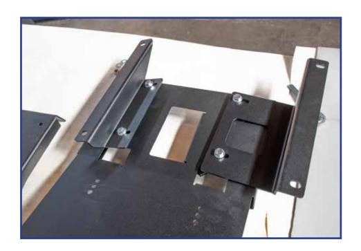
Place the camera/license bracket into position and secure with the stock bolts that came off from original door mount.
