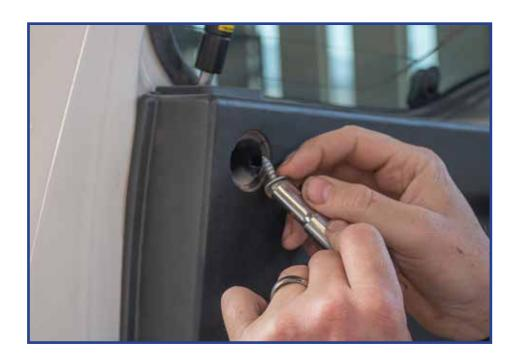
Once these are removed, you can now carefully pry the plastic panel away from the door starting from the bottom. We had to use a flat head screw driver at the bottom to get things started.
