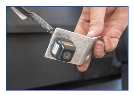
Once camera is secured to small bracket, you'll need to mount it to the bottom camera plate (see below). Secure with provided allen head bolts and nylon nuts. (see step 29 on next page)
