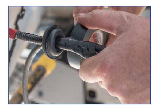
Here is how your wiring should look at this point. Go ahead and feed the original camera plug first and new wire back through the door and secure the rubber grommit to the door in its original location.
