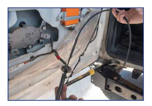
We used a bit of grease to help get the wire through the small opening of the rubber grommit.
