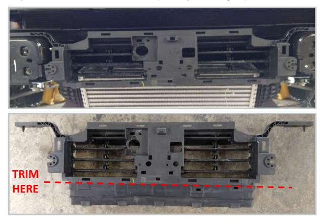
We will be rising the grille shutters for clearance. Drill in the location as shown (align on the vehicle if needed for location) to reattach to the OEM location and bolt size. Repeat for both sides.
