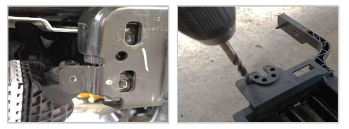
Mount the grill shutter back into place using the provided spacers and longer bolts on top and the new hole location with OEM hardware on the sides. Reconnect the wiring.
