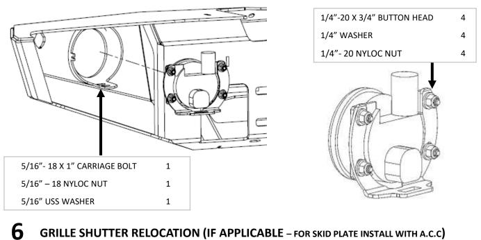
**GRILLE SHUTTER RELOCATION (IF APPLICABLE – FOR SKID PLATE INSTALL WITH A.C.C)** Detach the grille shutter as shown by disconnecting the wiring and 4 bolts. Cut off the lower plastic for clearance to reinstall the A.C.C (see skid plate install guide).
