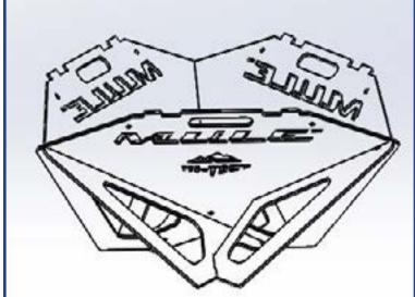
**3** D to ABC Place piece D onto top of pieces A, B, and C.
