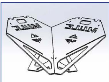
**2** C to AB Insert piece C into the slots of pieces A and B.
