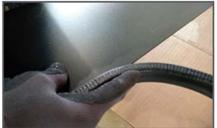
Install the weather stripping to the bottom of front fascia as shown and trim any excess.
