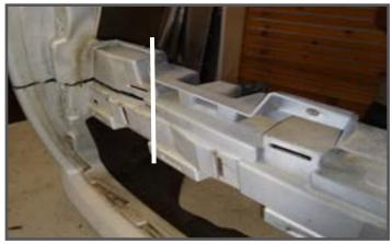
Cut the inside section of the bumper out on both ends.
