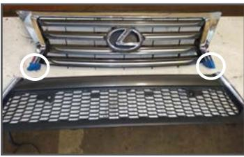
Trim back the ends (circled) to allow bracket and bumper clearance.
