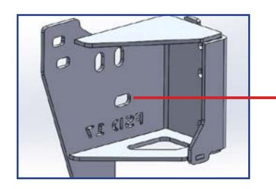
Drill hole into the frame in this location to fit a 5/8" bolt.
