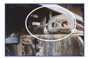
Save the hardware (bolt plates and nuts) from the original mounting area (circled) as these will be used to mount the brackets for the new bumper.
