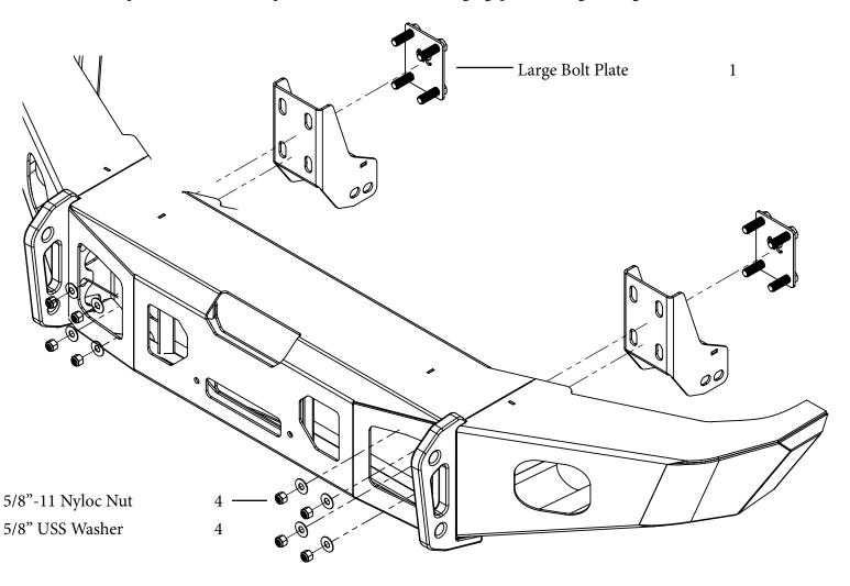
3/8" Hardware - Tighten to recommended 37 ft-lbs 1/2" Hardware - Tighten to recommended 90 ft-lbs 5/8" Hardware - Tighten to recommended 160 ft-lbs
