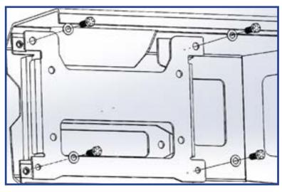
Attach 3/8" Clip Nuts to the Winch Mounting Plate Area
