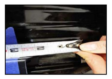
With the trim removed, start marking the mount locations by placing the tape measure at the end of the trim piece at the rear of the cab (circled below). From this point measure forward to the speficied dimensions below for placing the mounting brackets. Once located mark the hole locations for drilling and repeat for the other side of the vehicle.
