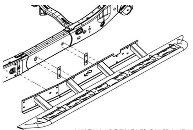
ALLIGN LARGE HOLES ON FRAME WITH HOLES ON ROCKER GUARD.
