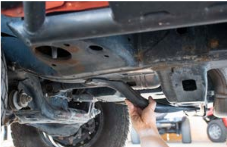
The curved bars shown left will also need to be removed with two bolts holding each one.
