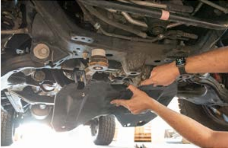
Mid section stock skid plate being removed.
