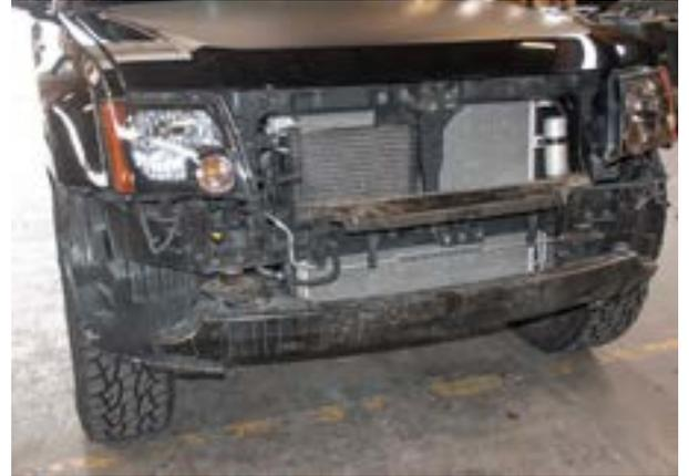
Remove frame piece as shown to right with the few remaining bolts that are holding it in place.
