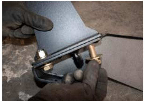
Line up the large frame bracket against the frame as shown with the 2 holes circled in photo. At this point you'll reuse the frame bolts that you initially removed to hand tighten the bracket into place.
