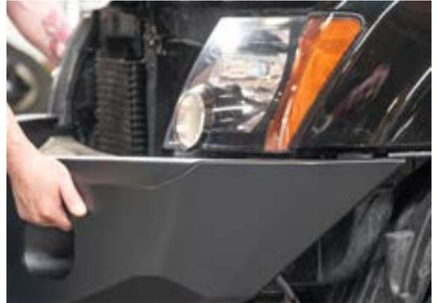
Carefully insert the provided frame bolts/washers into the frame holes with the bumper lined up. Secure with provided washers/nuts. If you're happy with bumper alignment, go ahead and tighten down all nuts and bolts on the frame brackets and the bumper.
