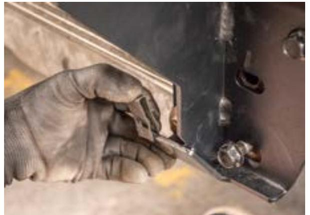
Carefully place bumper onto frame brackets and into proper alignment with body of vehicle.
