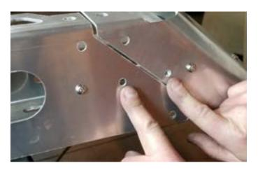
Make sure not to put any bolts in the holes pointed at below!
