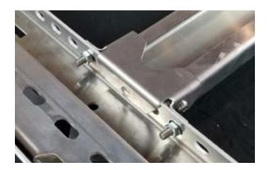
Flip over roof rack after all load bars are tightened down with tools and begin tightening all other rack bolts to prepare to mount onto vehicle.
