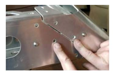
Next, attach reinforcement spacers as shown on all 6 hole locations with provided bolts & nuts. There are three mounting hole locations on each side.
