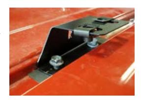
Once all mounts are in place, carefully place the roof rack onto the roof with a friend to line up with the mount brackets. Begin placing the provided bolts and washers into the front brackets first as these bolts are the same ones that also secure the bracket down into the roof rack. The rear use smaller bolts to secure the rack onto the brackets only.
