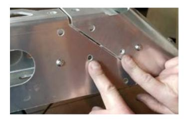
Make sure not to put any bolts in the holes pointed at below!
