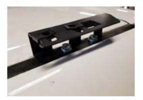
Once all mounts are put into place and tightened down, carefully place the roof rack onto the roof with a friend to line up with the mount brackets. Begin placing the provided bolts and washers into each hole and tighten down.
