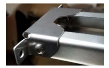
Flip roof rack on its back and attach load bars into desired locations as shown in photo. Using provided nuts and bolts, you may begin tightening down each load bar with two bolts/nuts for each side of load bars as shown.
