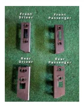
Peel off and place provided 3M strips, covering the holes as shown.
