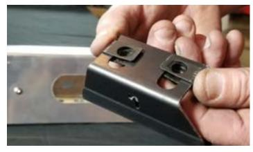
Once you've drilled out your roof holes around the vehicle and installed the riv nuts, place your mounting feet into position and tighten down into place with provided washers/bolts.
