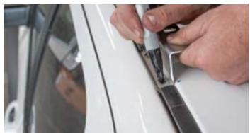
We recommend using a Center Punch tool to punch a small hole where you will be drilling so your drill bit doesn't slide out of place.
