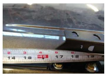
For the rear mounts, measure again from the start of the roof trim piece seam at the front of the vehicle (circled) to 61 1/4" for the front of the rear mount and 65 1/4" for the end of the rear mount. Placing the mounting bracket on the roof, and mark with a sharpie the ends of the mount where you'll need to cut the rubber trim. Verify the hole location before cuting and repeat for the other
