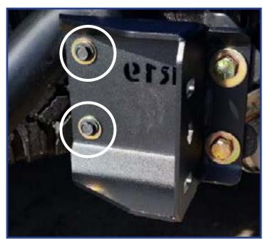
\*IF VEHICLE HAS A REAR DRIVERS SIDE STEP, YOU'LL NEED TO WIDEN THE 2 LEFT HOLES TO FIT THE 1/2" BOLTS.\*
