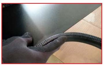
Install the weather stripping to the bottom of front fascia as shown right and trim any excess.
