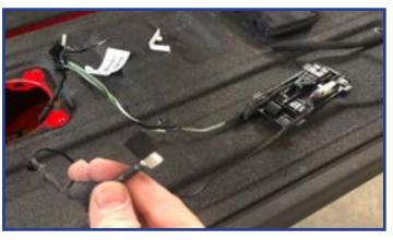
Now thread the wiring harness though the bottom of the tailgate and position behind the bumper, inserting the harness through the hole location in the license plate area.
