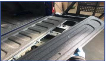
Different models may require remove the tailgate handle and other hardware. Next disassemble the OEM back up camera bracket and/or mounts, saving the hardware as it may be used in the new assembly. Some models will require the seperation of the wiring loom if they are connected to an electronic lock. Ram HD handle shown and Jeep Gladiator wire seperation shown below.
