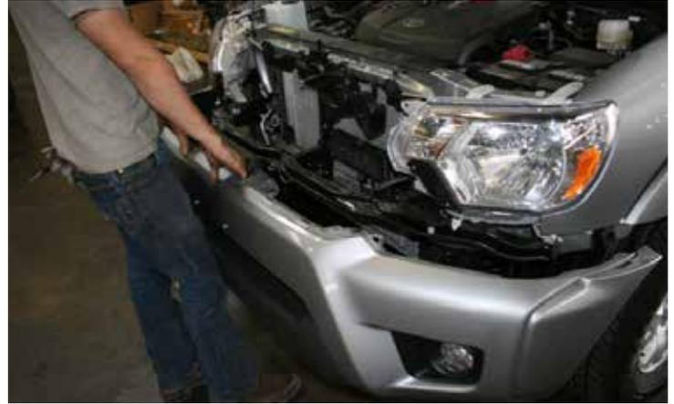
Next, you'll need to remove the internal frame piece below the headlight (See Fig 3B)
