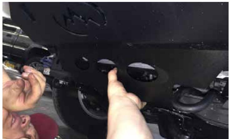
Secure the back end of the skid plate with existing stock bolts that are holding the stock skid plate onto the vehicle.
