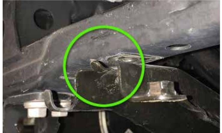
With the help of a friend, place the bumper onto the frame brackets and check for alignment around the front end. If spacing is fairly even from the bumper to the body of vehicle, go ahead and secure the front bumper to the frame brackets with provided hardware.
