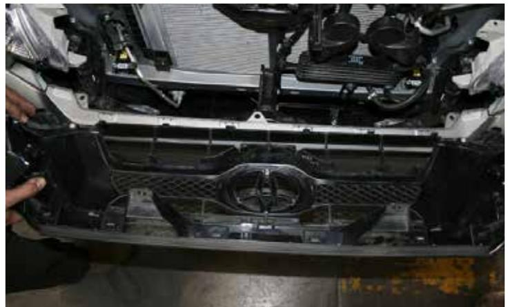
You will also need to use a socket wrench inside the front wheel wells to reach the bolt that holds the stock bumper on.
