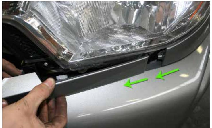
Shown is bumper being removed from the vehicle.
