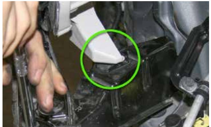
With a screwdriver, you'll also need to remove the black piece shown in Fig 4A / 4B
