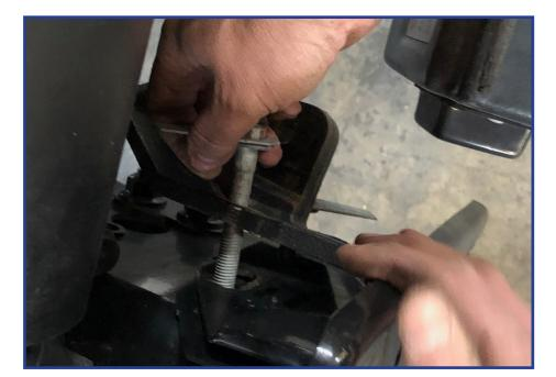
Remove all frame mount brackets from front of vehicle.
