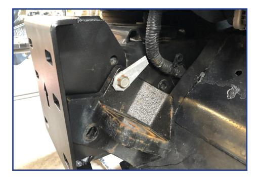
Hand twist nut on stock bolt to lightly secure mounting brackets.
