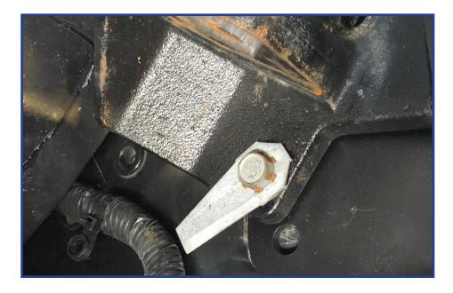
Once the winch has removed you can take upper bolt from frame mount.
