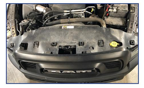
Remove stock grille face. Two screws located behind grille one passenger and driver side.
