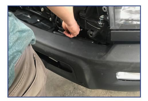
4 bolts are located next to headlights on both sides. 2 on upper portion of bumper and 2 on the lower.
