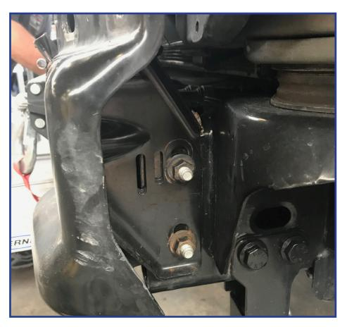
Remove lower bolt from winch frame bracket. This will allow the winch to swing slightly to the back. You can now unbolt the winch from the cast iron frame bracket and remove it from center of frame
