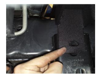
Using a 1/2'' bit, drill a hole through the 1st layer or sheet metal. Do not continue into the frame rail.
