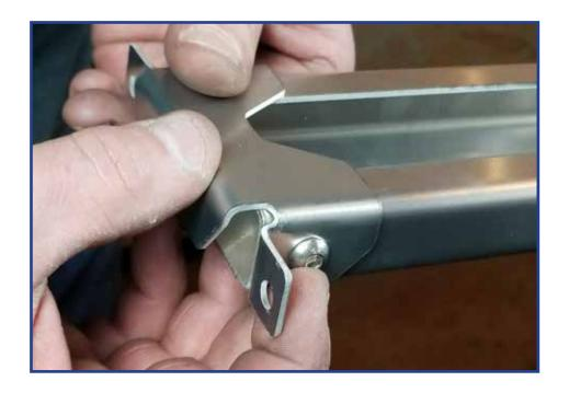
Flip roof rack on its back and attach load bars into desired locations as shown in photo. Using provided nuts and bolts, you may begin tightening down each load bar with two bolts/nuts for each side of load bars as shown.
