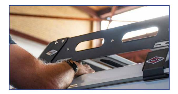
\*NOTE - for reference, here is where we positioned the rear end of the fascia and aligned all the gutter mounts to the rack in this position. Once happy with rack positioning, carefully take the rack back off and tighten all gutter mounts down securely.
