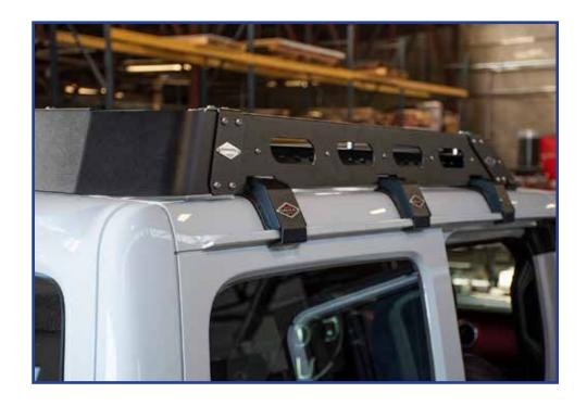
Once the rack is lined up with all gutter mounts, use the provided 1/2" bolts (2 for each mount). Hold the included nut retainer underneath for each gutter mount for the bolts to thread into from the top to secure the roof rack into its final position. (See example photo provided below)
