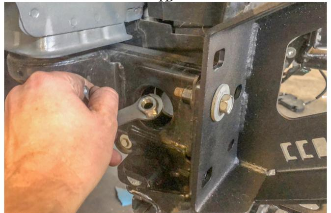
Slide in single nut retainer bracket into large hole in the back and tighten with bolt/washer as shown.
