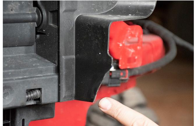
Using a flat head screwdriver or plastim trim removal tool, begin pushing the black grille frame away from the red cover.
