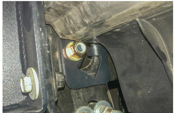
You'll then need to take the included bracket (2C) and place it on the inside of vehicle frame where the large bolt will go through (Fig 2A) and secured with washer and locking nut.
