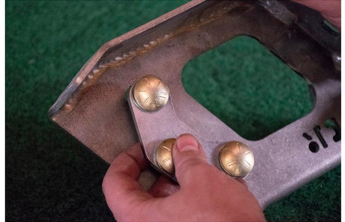
Shown right is the completed frame install (making sure all bolts are loose).
