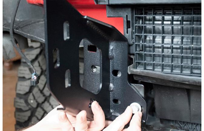
After hand tightening one of the stock bolts (See Fig 1B), you'll need to insert the provided bent nut retain-er for the 2nd bolt to thread to (shown in Fig 1C/)
