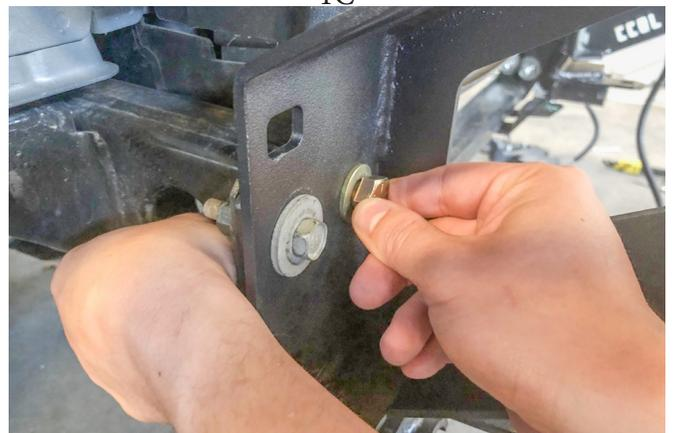
Next, you'll need to take the provided small back frame bracket and place it behind the large front bracket and against the vehicle frame.
