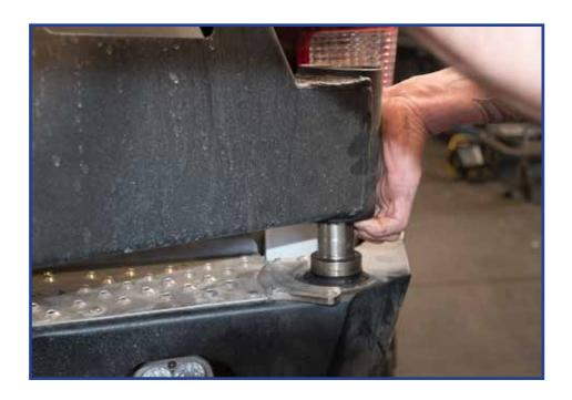
Once the arm is set in place on the spindle, grease the other bearing and drop it onto the spindle as shown below. Again, slide the arm back and forth and wiggle the arm if needed while pushing the bearing with your hand to make sure its set correctly.
