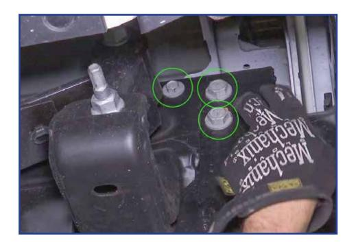
There is also one last bolt to remove on the passenger side shown below that will also need to be removed. \*Note - this bolt for the hitch receiver will need to be re-installed after the stock bumper comes off.
