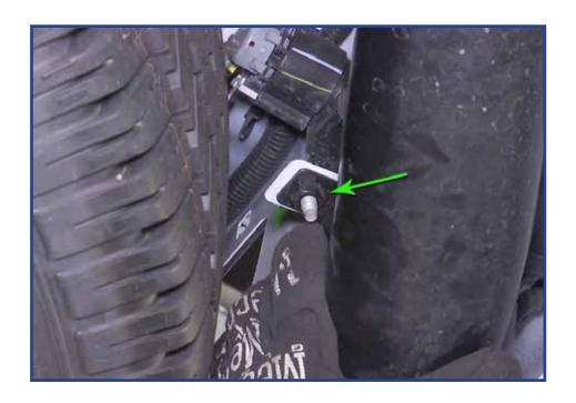
At this point we recommend disconnecting your trailer hitch plug either from underneath or through the license plate opening (see below). You'll need to pull up on the red tab and then it should disconnect.
