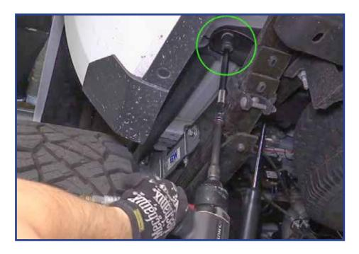
Next, we'll remove this bolt that is between the cab and the bed in the 'split' area shown below.
