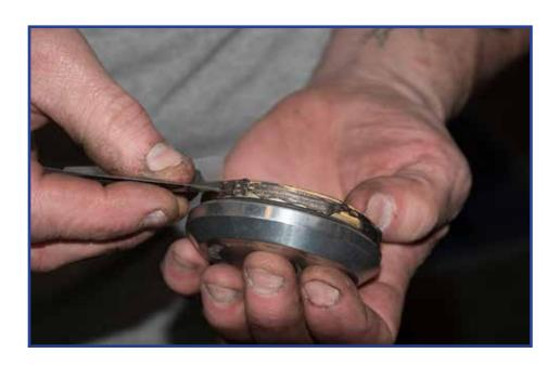
Place onto the spindle and hand tighten.
