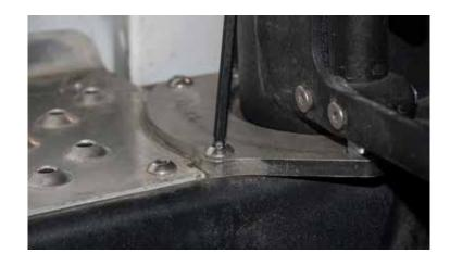
If handle needs to be adjusted, then these three bolts shown to right are the bolts you will need to adjust to do that.
