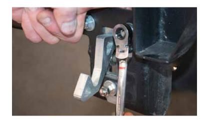
Shown to right are the additional bolts for the bump stop that can be adjusted for proper latching.
