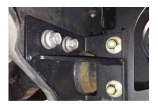
Adjust the bumper as desired then tighten all your bolts. We recommend tightening the top 2 socket cap bolts utilizing a hex key first...this will help the bumper from shifting as you tighten the rest of the bolts. It is also recommended you tighten the oem bolts on the mounting brackets last.
