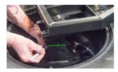
Flip arm over and position your tire mount into position. Tighten into place where you marked your lines.
