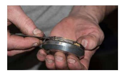
Attach cap onto spindle and hand tighten down.
