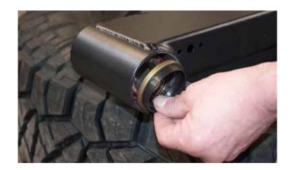
Place arm into position, holding the bearing/grease seal with hands, onto the spindle.
