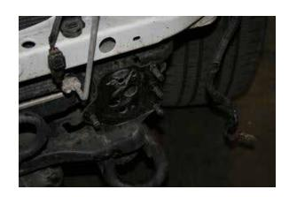
Center support bracket with has an extending mount coming off of it; this must be cut off in order for the bumper and/or winch to fit.
