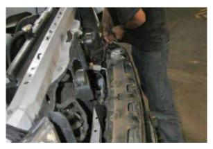
Remove the large metal bracket extending across the bumper with a 10mm socket and/or wrench.
