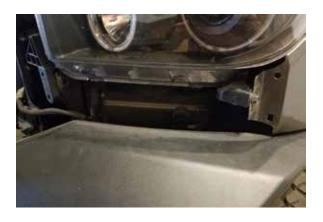
Remove inner fender well bolts on each side (pictured right).
