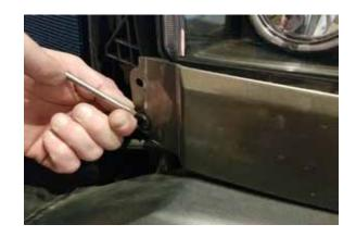
Once the panels are removed there are a series of 10mm bolts that need to be removed in order to remove the plastic of the stock bumper. They run along the front edge of the bumper just behind the plastic bumper edge and underneath the light.
