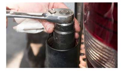
Open arm till the pin drops into place. If it doesn't as shown to right, you'll need to go to the next step below.
