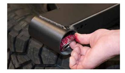
Now place grease seal as shown inside the bottom of the arm.
