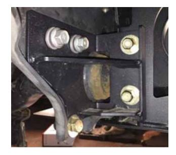
Adjust the bumper as desired, then tighten all bolts. We recommend tightening the top 2 socket cap bolts utilizing a hex key first.. this will help the bumper from shifting as you tighten the rest of the bolts. It is also recommended you tighten the oem bolts on the mounting brackets last.
