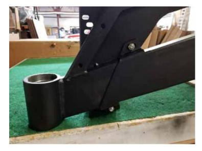
Use the last bolt, nut and washer and place through the top hole as shown in photo.
