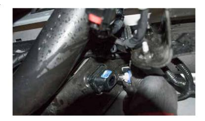
Remove receiver plug wiring from back of stock bumper.
