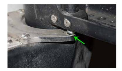
Adjust the button head bolts as shown until the pin drops into place. Then secure down again.
