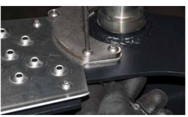
Lay the expedition one bumper on flat surface and begin prep work by attaching the skid plate to the bumper. Use button heads and bolts provided.
