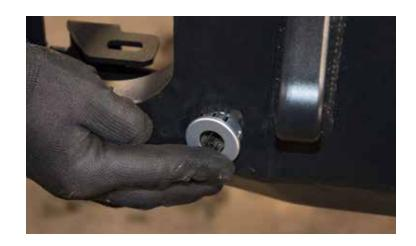
Fish your wiring harness through the bumper to attach sensor plugs.
