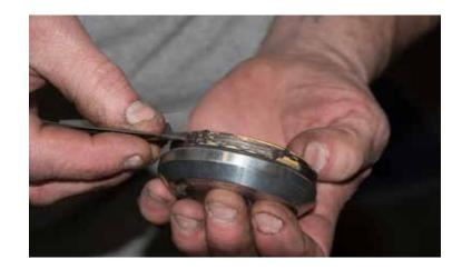
Attach cap onto spindle and hand tighten down.
