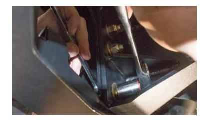
Lay your spare tire on the ground and set the tire mount into place. Now set the arm on top of it, marking the height when the arm is flat across it.
