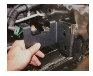
Depending on the bumper your installing with the pump you may want to locate the pump with the vacuum port facing forward. For example the Expedition One Trail Series full width bumper will have the winch mounted over the top of the vacuum pump in this instance the port facing foward is more ideal and potentially easier to get located. Also this will aleviate the need to possibly bend or manipulate the AC line for clearance.
