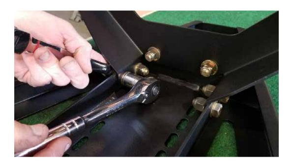
Attach tire mount bracket to desired position on front of mount
