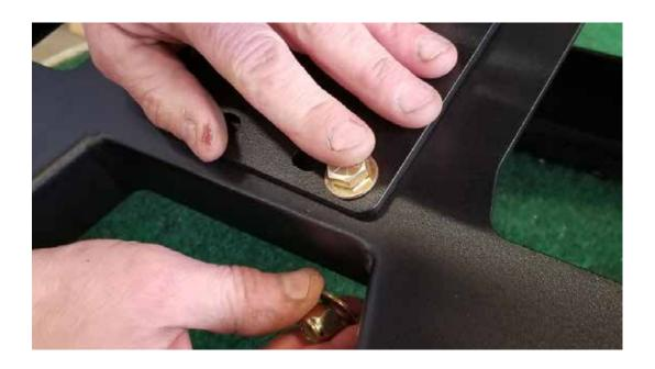
Tighten down all bolts with 9/16" socket wrench
