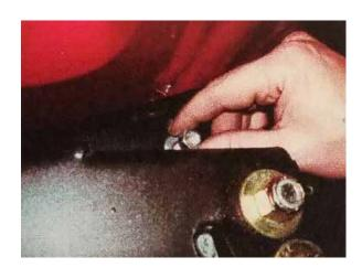
Install winch. Follow instructions provided with your winch. Make any needed adjustments to the positioning of the bumper. TIGHTEN BUMPER NUTS AND BOLTS. Then replace the plastic air dam.
