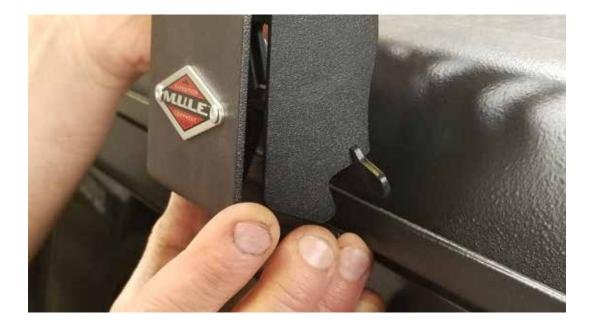
Using allen wrench, begin tightening your button head bolt into place.
