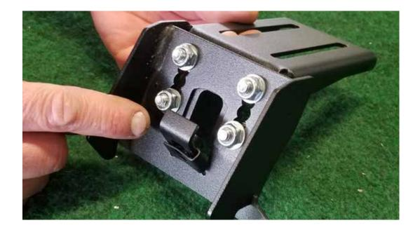
Reattach cover plate and use provided button head bolt to secure it in place. (Leave fairly loose to allow it slide over the gutter)
