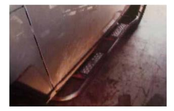
Lift the first slider and mount using the existing mounting holes in the frame and the 8 of the supplied M8 bolts and 8 flat washers.
