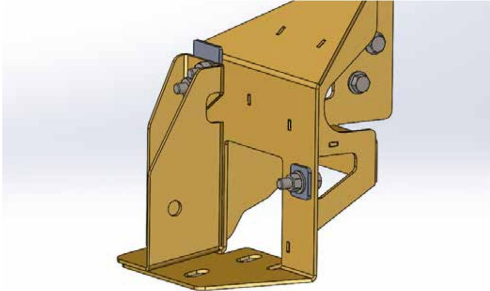
Use provided 1/2" bolts to attach your bumper onto the reinforcement brackets.
