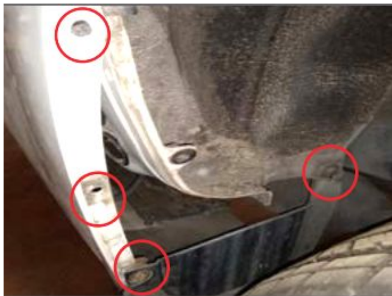
Wheel well panel (shown Removed) and hardware
