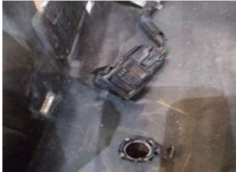
Disconnect the parking sensors from the bezels. Be care to not break any clips or parts of the bezel as they will be reused in the new bumper. Remove the bezels once the bumper is removed in step 2
