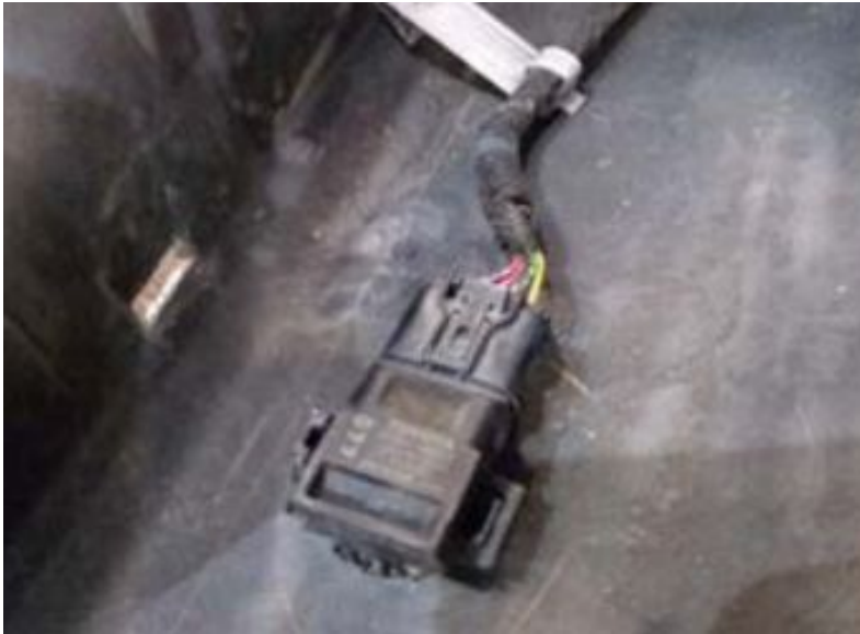
Disconnect the parking sensors from the bezels. Be care to not break any clips or parts of the bezel as they will be reused in the new bumper. Remove the bezels once the bumper is removed in step 2
