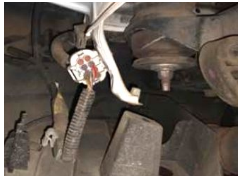
Disconnect all wiring harness connectors
