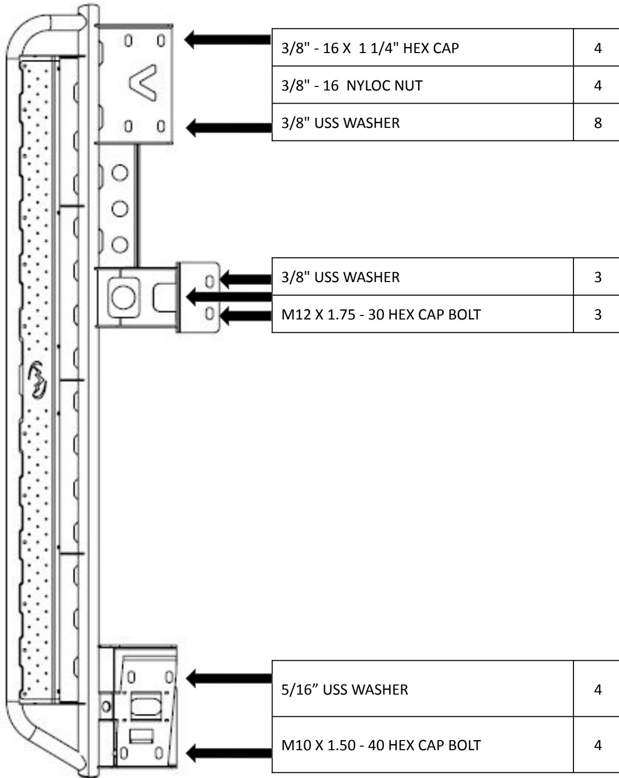
TIGHTEN ALL HARDWARE AFTER EVERYTHING IS INSTALLED ON THE VEHICLE. CHECK AND RETIGHTEN ALL HARDWARE AFTER THE FIRST 100 MILES OR AFTER OFF ROADING. CHECK REGULARLY AFTER EXTENDED OFFROAD USE
