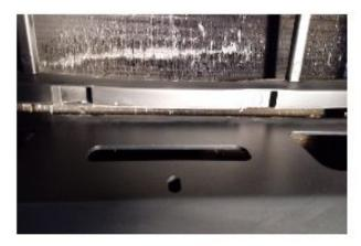
Now you can install the bumper, get the desired gap and start to tighten the bolts going side to side and increase the pressure. You will need to watch your gap while tighting the bolts.
