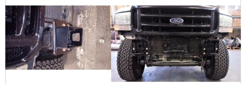
The clips that hold the bottom of the Grill on will need to be trimmed off. Undo the screws on top of the grill then pop the grill off so you can cut off the 2 center clip brackets, leave the outer two clips so your grill will still have a way to be attached.
