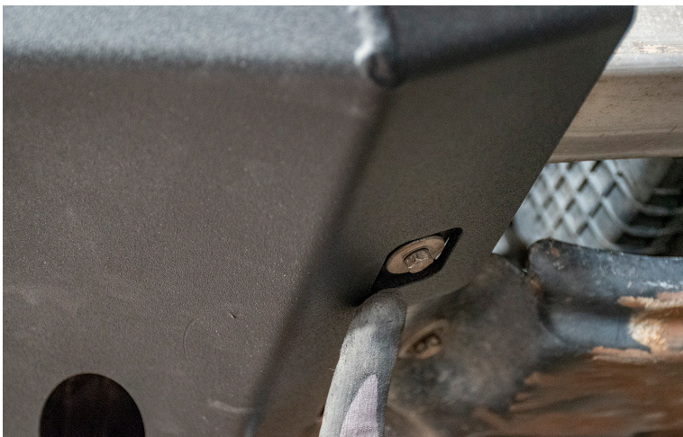
Install (2) bolts on bottom side to connect transition skid plate to bottom radiator bracket.
