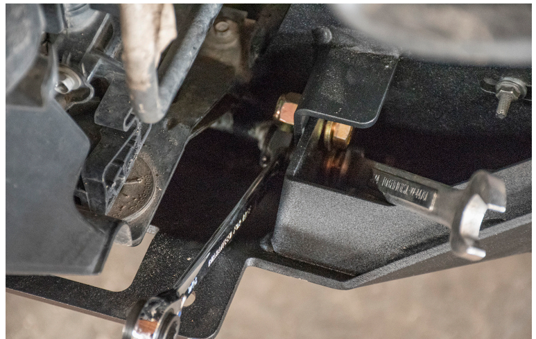
Install (2) bolts on bottom side to connect transition skid plate to bottom radiator bracket.
